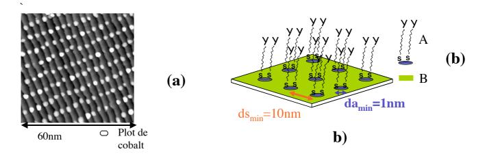
Figure 1 : scheme of the replication of the nanostructured network made of metallic islands (Co/Au (788)) in two interpenetrated molecular networks (molecules A and B)
